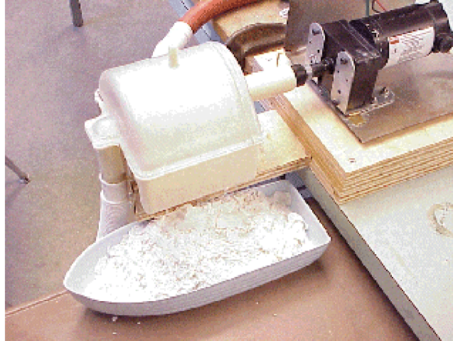
Dry cake discharge
